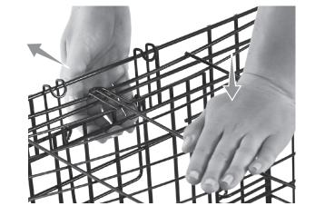
Crate sizes 42" and 48" have a "U-Wire" on the top panel that hooks over the end panel.
