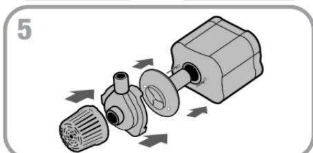
**Step 5.** Reassemble all pump parts and place in water before reconnecting to the power source.
