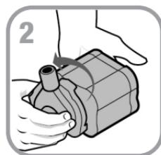
**Step 2.** Remove the impeller housing to expose the impeller assembly.
